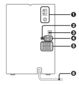
**1** AM LOOP jack and FM 75  $\Omega$  terminal (4) Plug in the supplied AM and FM antennas.
